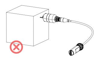
Incorrect installation: Placement close to the slab top. Prongs partially outside the substrate.
