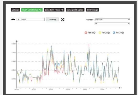
Progression of short-time flicker Pst during a day via the device website
