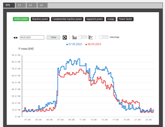
Daily load profile with previous day values for a PME sensor via web page of the base unit
