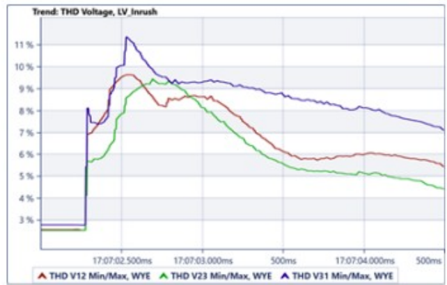
LV side Power Quality recordings – Building #1 UPS upstream
