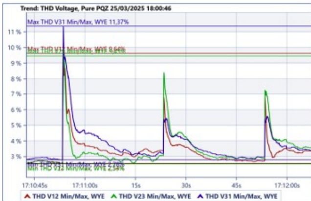
LV side Power Quality recordings – Building #1 UPS upstream
