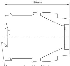
Snap-on mounting on 35 mm DIN rail to EN 60715
