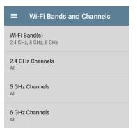
**Note:** Selecting a subset of channels and bands lets you exclude scans of unneeded channels from the survey. This improves survey performance and reduces the amount of data collected.
