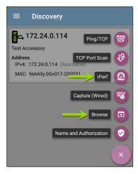
Select the iPerf app button to open the iPerf app with the IP address populated from the Test Accessory in Discovery.
