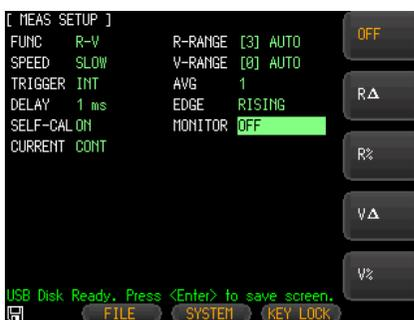
3. Use option key on the right of the LCD screen to select a monitor parameter or turn off monitor function by pushing OFF button.
