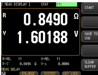
2. Press the **START** option key on the right of the LCD screen again to restart the statistics logging function.
