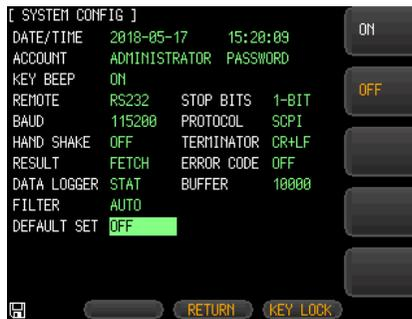
4. Press **ON** and then YES option key on the right of the LCD screen to change setting.
