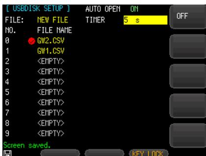
11. Enter a number from key pad, then press “s” option key on the right of the LCD screen to set interval time for recording measurement data.
