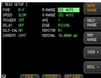
5. Use option key on the right of the LCD screen to select a desired measurement range.
