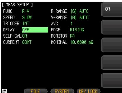
3. Use option key on the right of the LCD screen to turn on delay timer function.
