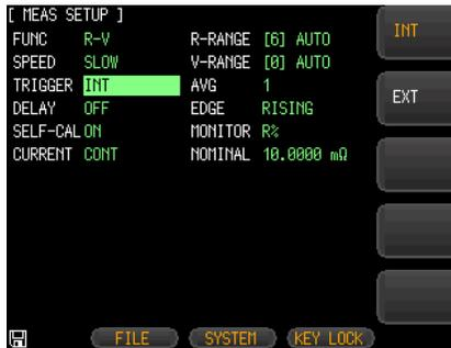
3. Use option key on the right of the LCD screen to select a trigger mode for this measurement item.
