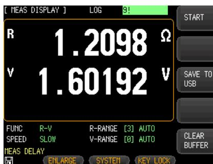
2. Press the **START** option key on the right of the LCD screen again to restart the data logging function.
