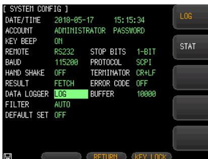
4. Press the **LOG** option key on the right of the LCD screen.
