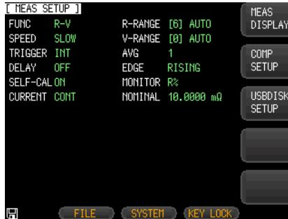
2. Press the **MEAS DISPLAY** option key on the right of the LCD screen. The MEAS DISPLAY page will display on the screen.
