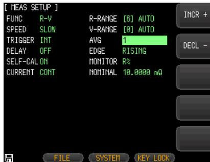
3. Use option key on the right of the LCD screen to increase or decrease average measurement frequency.
