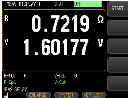
2. Press the **START** option key on the right of the LCD screen to start statistics function. The statistics of data will keep running until the number of setting buffer is up.
