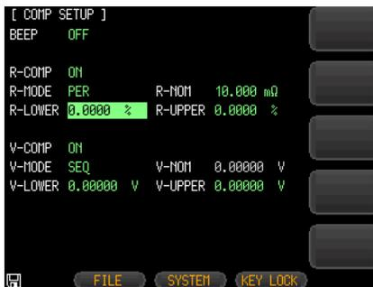
9. Use key pad to input upper and lower limits values and option key on the right of the LCD screen to select corresponding resistance and voltage unit.
