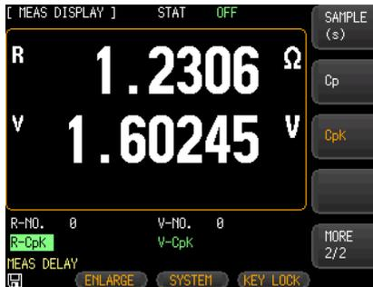
3. Use option key on the right of the LCD screen to select desired statistic parameters
