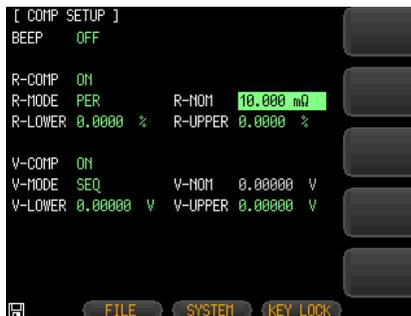
7. Use key pad to input normal value and option key on the right of the LCD screen to select corresponding resistance and voltage unit.
