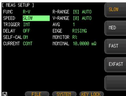
3. Use option key on the right of the LCD screen to select a test speed for this measurement item.
