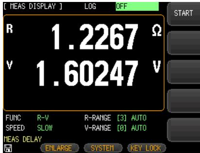
2. Press the **START** option key on the right of the LCD screen to start continuous data logging function. The data logging will keep running until the number of setting buffer is up.
