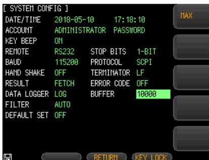
4. Enter a number from key pad, then press Enter key or press MAX option key on the right of the LCD to set up the number of data for logging.
