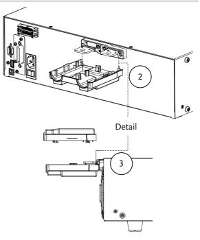
4. Use your thumb to slide the terminal covers shut, as shown in the diagram below.
