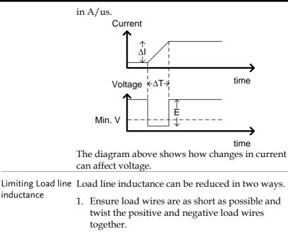
2. Current change can be limited by limiting the slew rate or response speed when switching in CR and CC mode.
