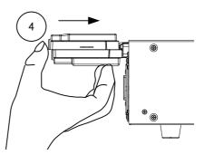
5. When the top and bottom covers are flush, reinsert the screw that was removed in step 1.
