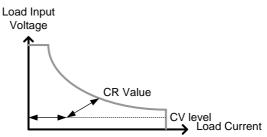
Note that when the source voltage is less than the CV level, no current will flow due to a very high impedance.
