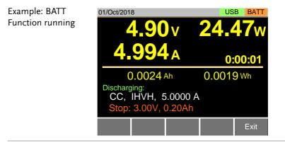
Results: Battery stop Voltage or stop time or stop AH tripped
