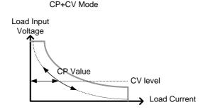
Note that when the source voltage is less than the CV level, no current will flow due to a very high impedance.
