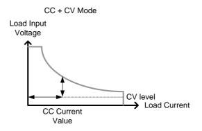
Note that when the source voltage is less than the CV level, no current will flow due to a very high impedance.
