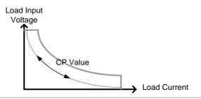
CP+CV Mode When CP+CV mode is enabled, the unit will act as a constant power load after the input voltage is greater than the user-defined CV level. At the CV level, the unit works as a constant voltage load. This mode effectively creates a voltage ceiling before the unit operates in CP mode. The diagram below illustrates this.
