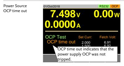
OCP time out will occur if the power supply's OCP fails to trigger. This is determined when the measured voltage is less than Trig V and the measured current is greater than End C.
