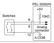
The range can only be externally controlled when the IRange has been set to High using the front panel controls.
