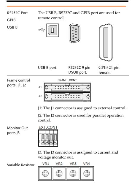
The variable resistors are used to adjust the full scale and offset setting for the input value of the external control sources such as voltage or resistance.
