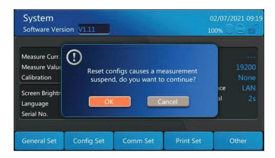
Select [System reset], the following dialog box will pop up. System reset requires clearing local memory, configuration and statistics. System reset also initializes the data saved in the panel:
