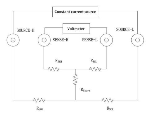
RSEH and RSEL are wiring resistances for SENSE-H and SENSE-L
