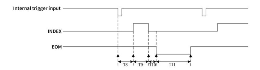
HOLD mode outputs EOM width and measurement mode after calculation is completed; PULSE mode outputs EOM after calculation is completed, and cancels EOM after keeping the set pulse width time. Time parameters are shown in the following table.
