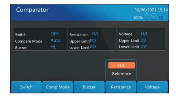
Enter [0.2] in [Upper limit], click the up and down keys to adjust to the lower limit input box, and enter [0.05]. Click [Enter] to complete the setting. The values after setting are as follows:
