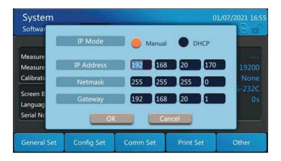
After it is set, press the up and down direction keys to select [Confirm] setting, or select [Cancel] setting, and then click [Enter] to complete the setting.
