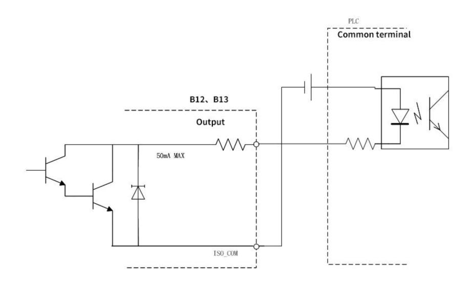
• Connection with PLC input (positive common terminal output)
