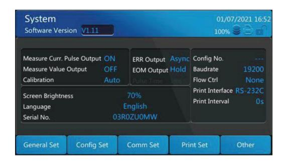
The ON/OFF of measurements output, automatic/manual calibration setting, ERR output asynchronization/synchronization, EOM output, etc. are operated according to this operation mode.
