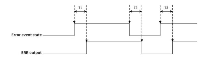
ERR asynchronous output timing
