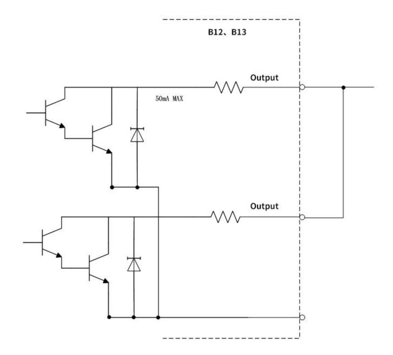
• Connection with PLC input (negative common terminal output)
