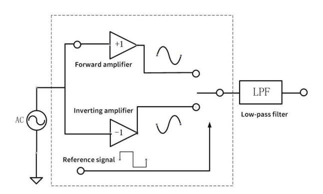
Set the AC current reference signal generated by the instrument as V1, and set the signal voltage for synchronous detection as V2, so that:
