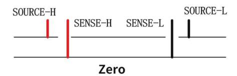
When using pin type test line for zero setting, please connect the test line as shown below.
