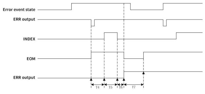
ERR synchronous output timing
