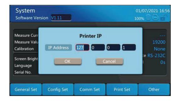
Then the setting of print interface as network interface is completed.
