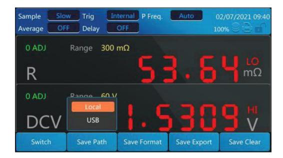
Insert the USB flash disk, click [F2X] key continuously to select [USB], and click [Enter] to complete the setting of storage path as USB.
