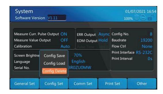
Select [Configuration deleting], the configuration number input box will pop up, fill in the configuration number to be deleted, and click [Enter],
