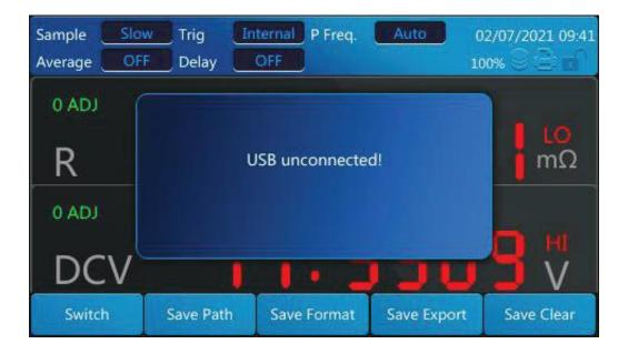
After inserting the USB flash disk, click [F4] to select data transfer format, and click [Enter] to confirm:
