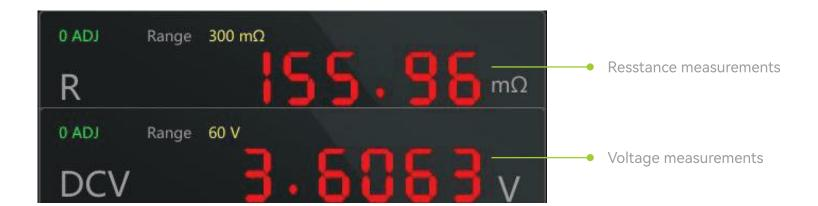
When  $[\Omega]$  function is selected, the measurement screen only displays the resistance measurement.
