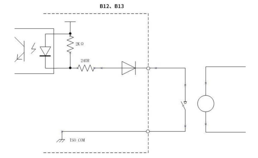
• Connection with PLC (negative common terminal output)
