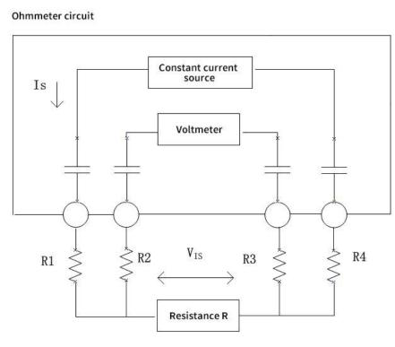
Resistance of R1~R4 test line and contact resistance of contact part
