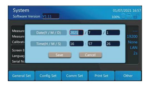
Press the left and right direction keys to switch the input box, and press the up and down direction keys to select settings or [Save] and [Cancel] keys. After it is set, you must press [Enter] key to confirm, otherwise the setting is invalid;
