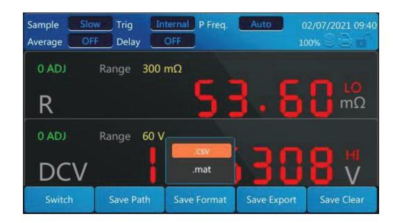
On the storage page, press [F3] continuously until [.mat] is selected, and then click [Enter] to complete the setting of storage format as [.mat].
