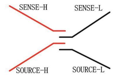
When using pin type test line for zero setting, please connect the test line as shown below.
