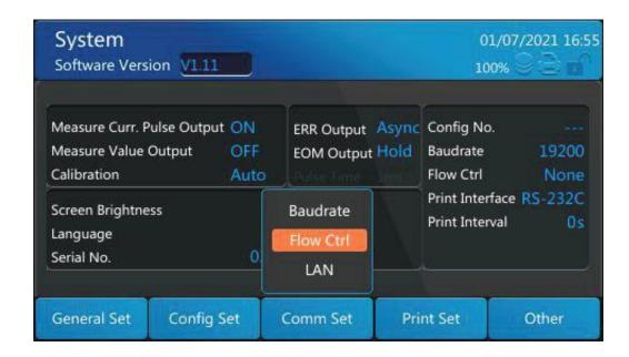
Press [Enter], the flow control submenu will pop up, and press [F3] to select the value.
