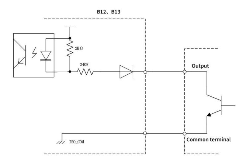
• Connection with PLC (positive common terminal output)
