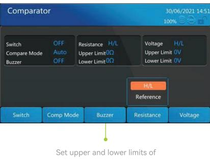
Set upper and lower limits of Set upper and lower limits of voltage and reference value range resistance and reference value range
