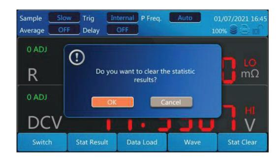
When the number of statistical packets is 1,000, clear the last statistical results and carry out the next statistics. If the number of statistical packets is less than 1,000, continue to carry out statistics following the number of statistical packets last time.
