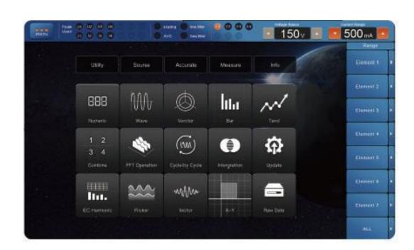
The major measured items and parts of functions commonly used can be displayed on the main menu in the form of icons, which you can press and select to access to the corresponding menus easily. If want to go back to the previous menu, you can press the Menu icon again. The element ranges are displayed in the context menu at the right side of the main menu.
