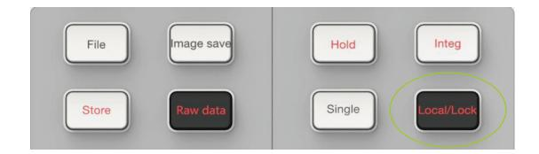
If you perform the operations according to the Procedure 2, not only the screen will be locked, but also the press keys on the panel except the Power key are all locked, indicator of the LOCAL/LOCK key illuminated. Only when you press and hold the LOCAL/LOCK key on the panel again for 3 seconds can the press keys on the panel and the touch screen be unlocked to be used again.
