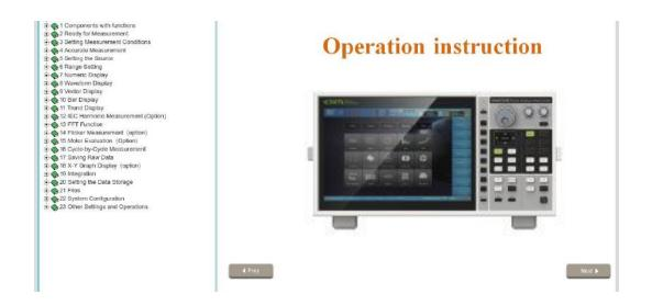
When you click any function (such as INTEG, STORE) in the HELP interface except <Help> key, you can access to the corresponding contents of descriptions and explanations. At the same time, you can use the arrow keys (up/down/left/ right) and the "Enter" key r to select in the catalog of help document for related descriptions.
