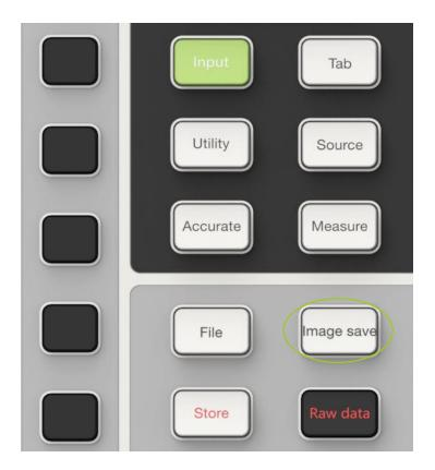
2) Function: The screen image can be saved in this instrument.
