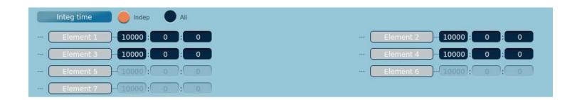
The selected unit can be set in the integral time, while the unselected unit cannot be set in integral time.
