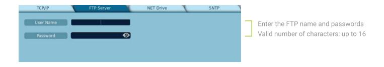
You can access this instrument from a PC via FTP server.
