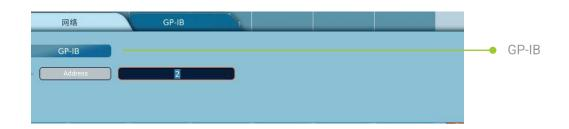
3) Set GP-IB address of the instrument, connection and data transmission between the computer and the instrument.
