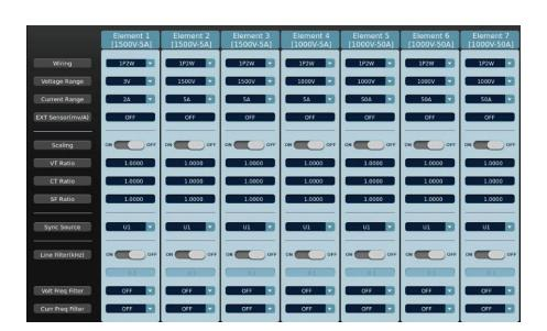
The contents listed in the parameter list include voltage and current information of each input element module. Parameters that can be set include the wring systems of each unit, voltage range, the current range, external sensor, scaling, VT ratio, CT ratio, SF ratio, synchronization source, line filter, voltage frequency filter and current frequency filter, etc.
