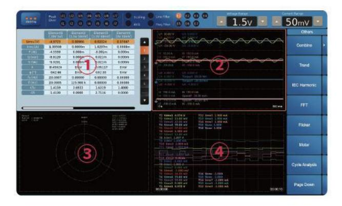
Click on the "Combine" menu, select several types of data to be shown on the screen. If you select the display types such as the waveform, numeric, vector graph and bar graph, they will be all displayed on the screen. The TAB key allows you to switch between menus to set the data to be displayed.
