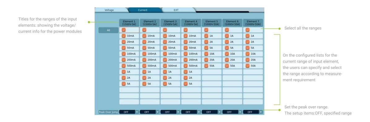
The options of current range vary depending on different module. For the specific range, please refer to "6.1 Setting fixed range of the voltage and current".
