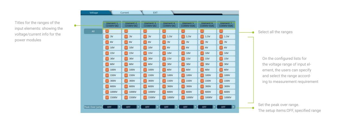
The options of voltage range vary depending on different module. For the specific range, please refer to "6.1 Setting fixed range of the voltage and current".
