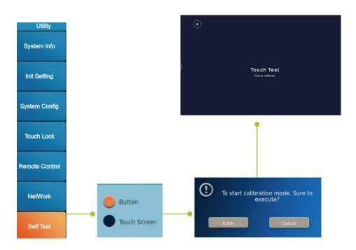
There are 5 calibration locations(in sequence are top left corner, top right corner, bottom left corner, bottom right corner, middle) on the calibration screen. Each time when you click anywhere on the touch screen, the calibration locations/ points will appear then disappear in sequence.
