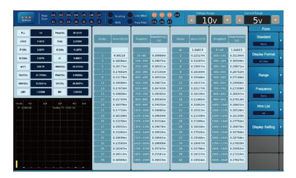
By default, the data information regarding power spectrum, Hrm/InterHar sub Group and Hrm/InterHar State can be displayed simultaneously on the IEC display menu.
