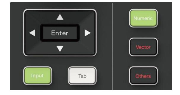
The parameters can be set by the cursor: You can move the cursor to the option and then press ENTER key, select or edit appropriate parameters in the drop down menus, and then press ENTER to confirm the parameters.
