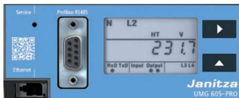
Fig. UMG605-PRO with Profibus interface.
