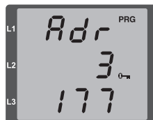
Fig. TCP / IP address, byte 3, value 177
