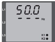
Fig. No rotation field direction detectable.
