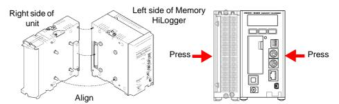
Secure the unit in place with the connection fittings at the top and bottom of the unit.
