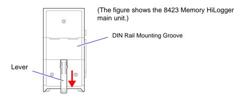
Hook the hooks at the top of the DIN rail mounting groove on to the DIN rail and push in the bottom.
