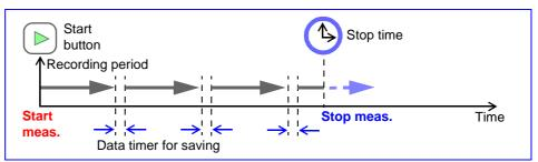
When measurement stop time is set within recording period for timer measurement
