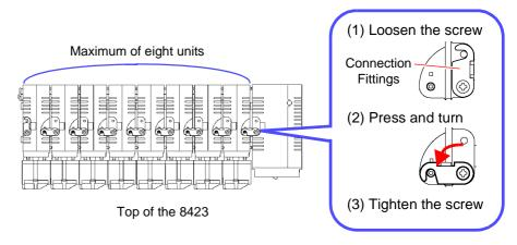
4. Attach the supplied connector cover to the unit on the very left side when looking from the front.
