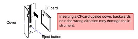
Fully insert the CF card from the front with the top surface facing left (cover side), and then close the cover.
