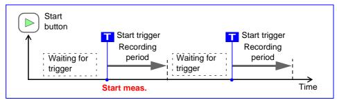
When stop trigger is set and stop trigger is applied before recording period
