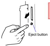
Do not remove the CF card while the CF card access LED is lit. The files of the CF card will become unreadable, and recording will no longer be able to be performed properly.
