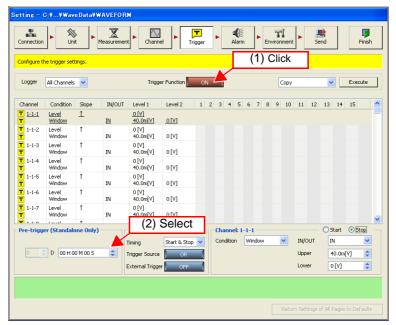
3. Set the pre-trigger. Enter the time to apply the trigger.
