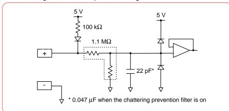
Model 8997 Alarm Unit Output Circuit Diagram
