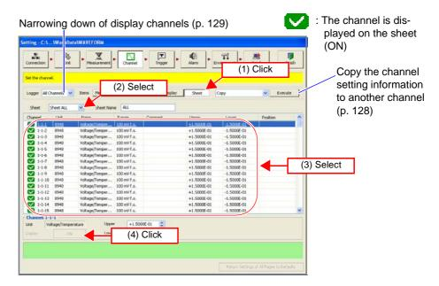
In the case of the 8948 Voltage/Temp Unit, 8949 Universal Unit, and 8996 Digital/Pulse Unit (input type: pulse), set the upper limit and lower limit of the screen display.
