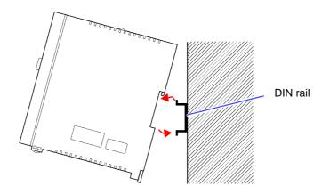
**5**. Push up the levers until they click into place. When you want to unmount the instrument from the DIN rail, perform the mounting procedure in the reverse order.
