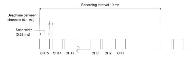
When the digital filter is off, the scan widths and dead times between channels are fixed to the values shown in the figure above regardless of the recording intervals. When the digital filter is on, the scan widths and dead times between channels vary in accordance with the recording intervals.
