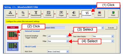
2. Set ON or OFF for the filter of the signal of each of the SMPL/TRIG, START, and STOP inputs of the external control input terminals.
