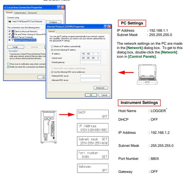
When connecting one PC and one instrument by the conversion connector of the 9642 LAN CABLE, the IP address can be specified arbitrarily, but there is no problem with using a private IP address.
