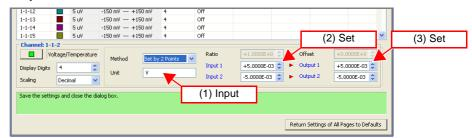
6. If the setting method is "Setting Method 1," set the physical quantity per pulse.
