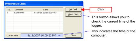
Depending on the timing in which the time is set, an offset of up to ± 1 second may be generated between Logger Utility and the 8423 main unit.
