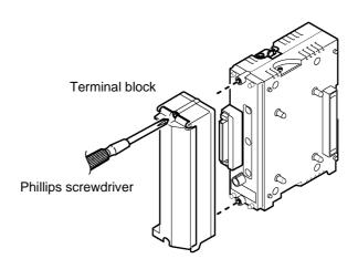
3. Connect the cable, and then attach the terminal block by performing the procedure up to now in the reverse order.
