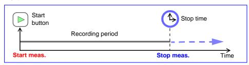
When measurement start time is set for timer measurement and stop time is set after recording period
