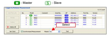
4. Click the [Test] button to display the synchronization test result.
