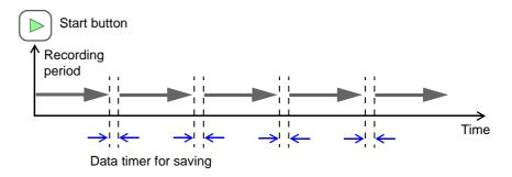
If you set a repeat measurement interval for timer measurement, it is possible to repeat measurement while leaving a gap at a fixed interval as shown in the figure below.
