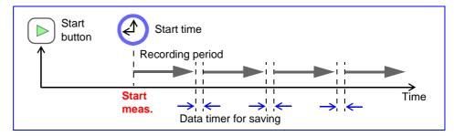
When measurement stop time is set after recording period for timer measurement
