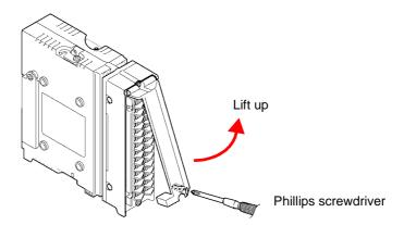
Loosen the screws of the terminal block, connect the input cable, and then tighten the screws.
