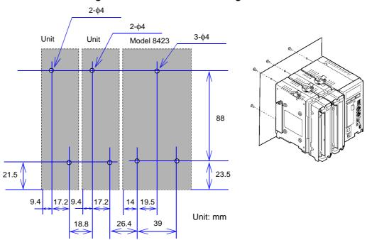
3. Insert the screws from the back side of the wall surface and secure the instrument with the nuts on the rear of the instrument.
