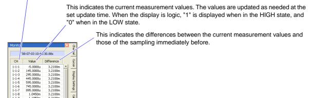
If there is no data for the low-speed unit at the latest position during dual sampling, the last measured data is displayed. In such a case, the character background is gray.
