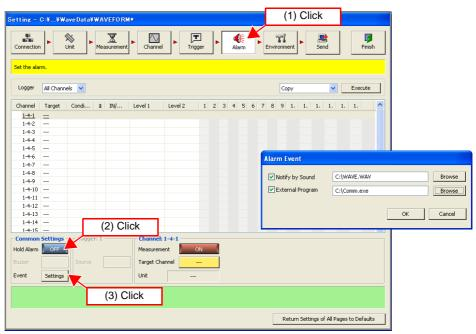
Alarm Hold: This sets whether to hold output when the alarm condition of a certain alarm channel is satisfied, and the alarm is output.
