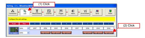
When simultaneously measuring different physical quantities, you can reduce the amount of data compared with measuring using normal sampling by selecting "High Speed" for high-speed phenomena such as voltage, and selecting "Low Speed" for capturing phenomena with gentle variations such as temperature and humidity.
