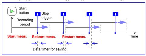
When start trigger is applied during timer measurement and stop trigger is applied before measurement stop time
