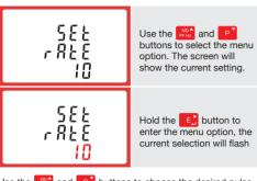
Use the price and price buttons to choose the desired pulse rate. To save the new setting, hold the button for 3 seconds until the selection stops flashing
