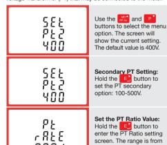
The PT Rate is the PT Primary divided by the PT Secondary. For Example: Voltage Transformer - 11000÷110=100, so the PT Rate would be 0100 and the PT2 would be 110.
