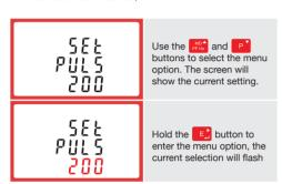
Use the policy and buttons to choose the desired pulse rate. To save the new setting, hold the seconds until the selection stops flashing
