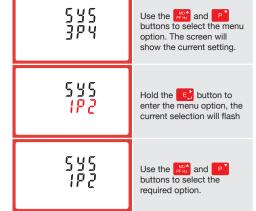
Hold the button to confirm your adjustment. Hold th button for 3 seconds to exit the set up menu.
