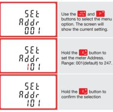
Use the press the buttons to choose the necessary number, then press the button to move along to the next number. To save the new setting, hold the button for 3 seconds until the selection stops flashing
