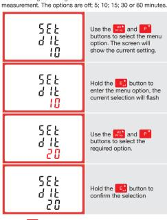
Hold the WA button for 3 seconds to exit the set up menu.
