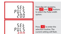
Use and buttons to choose pulse width. On completion of the entry procedure press [ to confirm the setting and press 2/14 to return to the main set up menu.
