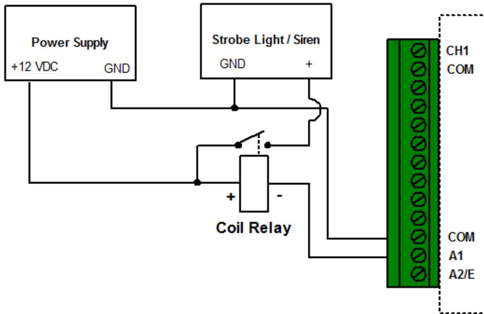
**Alarm1 is used as switch of the power supply.**
