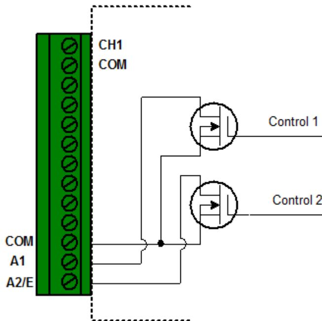
Alarm1 and A2/EXT can be associated with alarm state and/or excitation control. Please refer to Alarm Output and Excitation Control for details.
