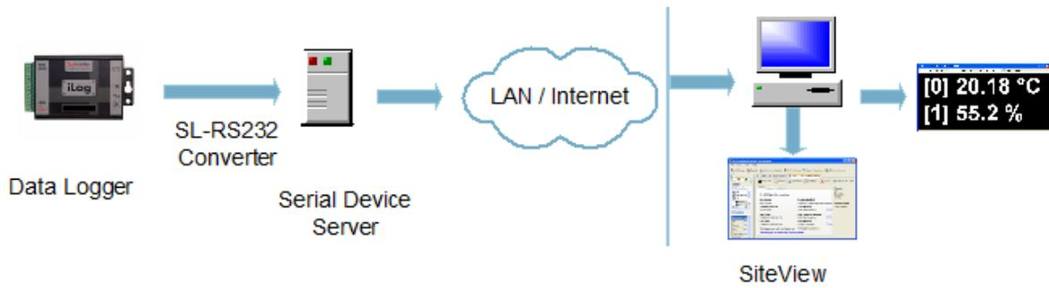
**Ethernet Connection (with Ethernet – Serial Converter)**
