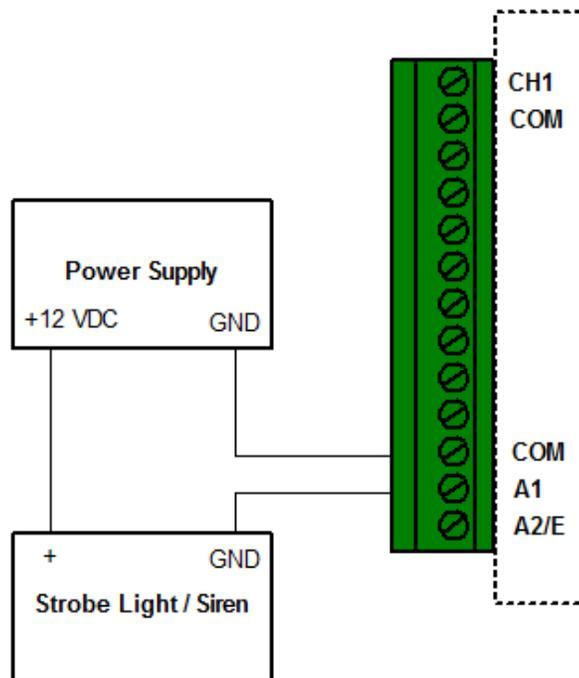
**Alarm1 is used as switch to turn on/off siren based on alarm state.**
